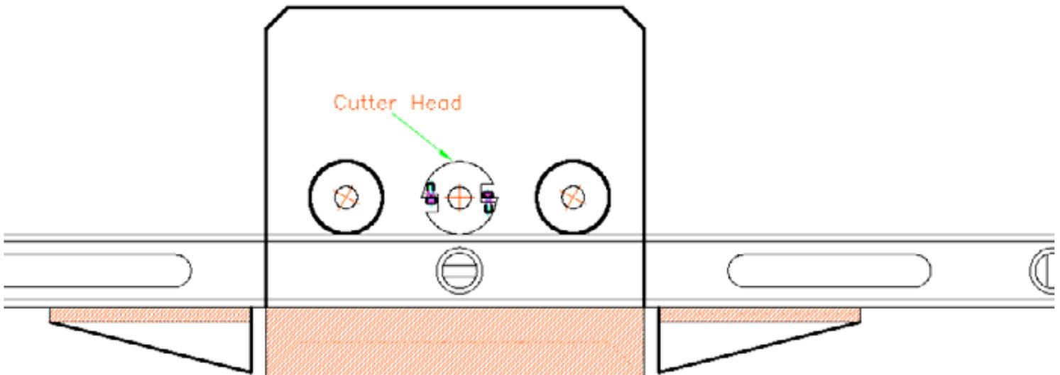
Step 5: Lower the cutter head assembly until the feed rollers hold the straight edge firmly in place.
