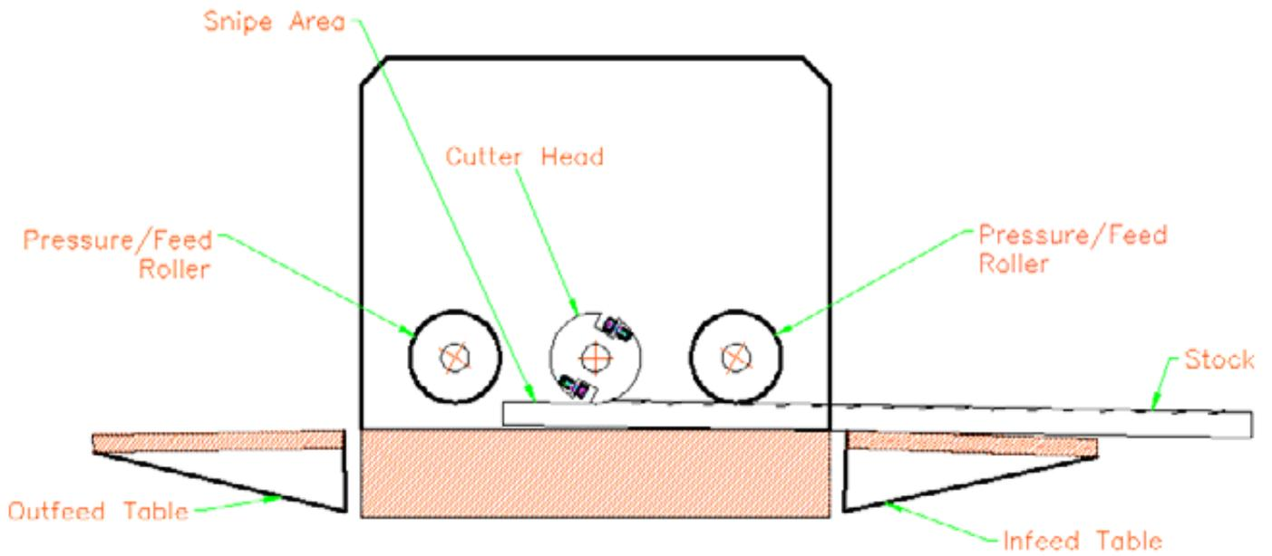
The proper setup will apply some pressure on the extremes of the stock as it travels through the planer. This should result in snipe free planing.
